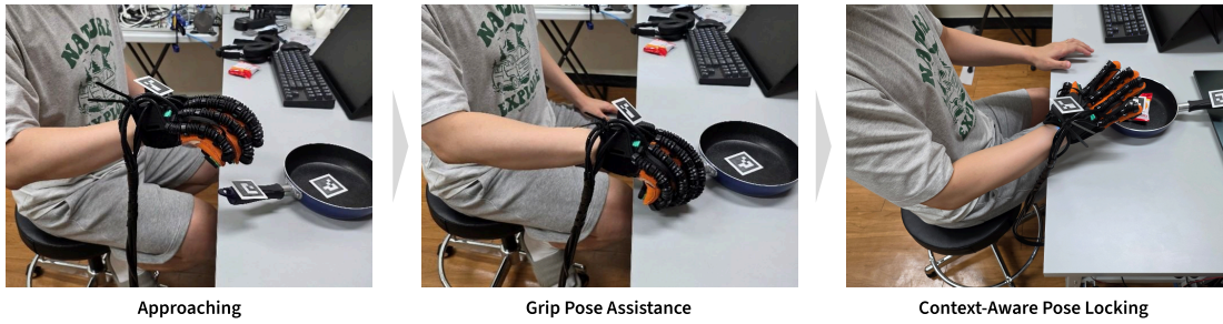
Figure 11: Overview of experiment 2. Depending on motion trajectory toward the frying pan, different poses are assigned to assist or inhibit subsequent actions.
