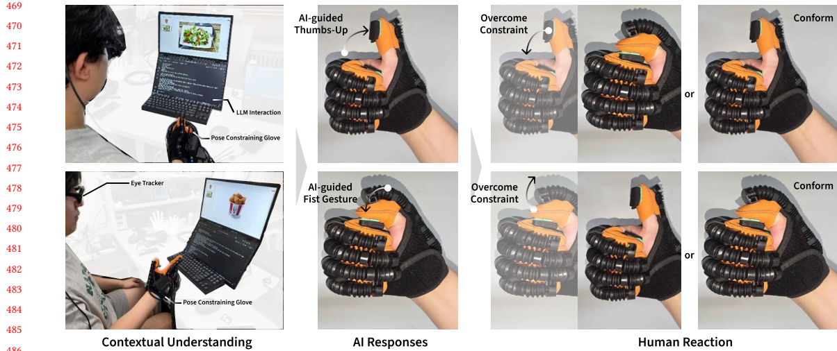
487 Fig. 5. Overview of Experiment 1. Poses transmitted from AI agents are illustrated. Then, there are basically two options for users, 488 either overcome or conform to the constraint. The gradient-arrows indicate start (white) and end (black) of a motion. 489
