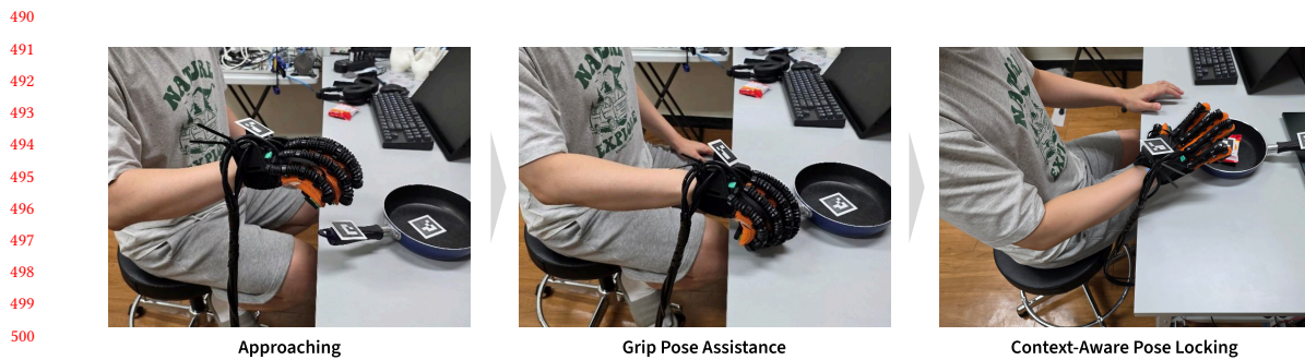
502 Fig. 6. Overview of Experiment 2. Depending on motion trajectory toward the frying pan, different poses are assigned to assist or 503 inhibit subsequent actions. 504 505
